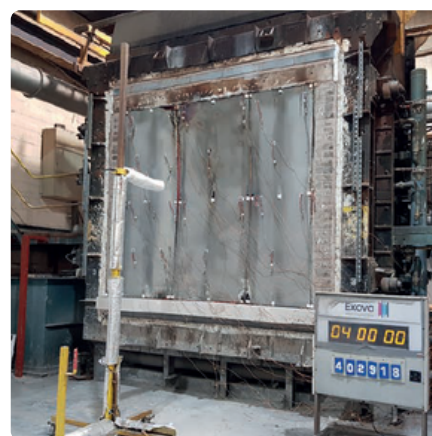
Third party, bi-directional fire testing to ensure fire integrity
